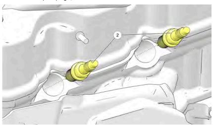
3. Reverse the procedure for spark plug installation. Torque to specification.
