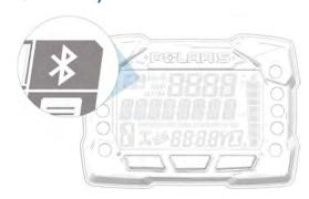
If you are browsing any of the Bluetooth® menus and the vehicle starts to move faster than 2 KPH, the menu will automatically display *VEHICLE MOVING*. If you attempt to access Bluetooth® menus while the vehicle is moving faster than 2 KPH, the screen will display *VEHICLE MOVING* momentarily, and then it will redirect to the options menu.
