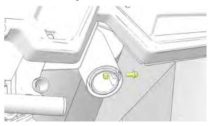
3. Remove the arrestor from the end of the muffler.
