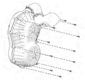
7. Using care, pull the outer PVT cover out the left rear wheel well.
