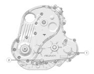
The fill plug is located on the right side of the ATV behind the footwell. The drain plug ② is located on the bottom rear side of the gearcase.
