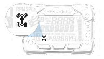
The All Wheel Drive (AWD) system is controlled by the Driveline switch. Engage AWD before getting into conditions where front wheel drive may be needed. If the rear wheels are spinning, release the throttle before switching to AWD.
