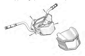
2. Unplug the headlamp from the wiring harness. Be sure to pull on the connector, not on the wiring.
