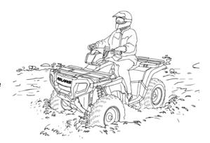
4. After leaving water, test the brakes. Apply them lightly several times while driving slowly. The friction will help dry out the pads.
