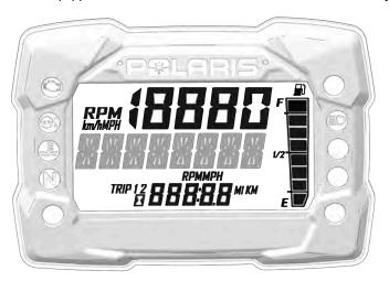
To toggle through available features, press Reverse Override / Mode Button ① from the left hand controls. For the full list of available features, see the Display Area 2 section of this chapter.
